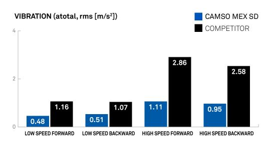
Throughout the entire test, the vibration level was 42% lower with the Camso tracks than the OEM quality track regardless the speed and the direction.
